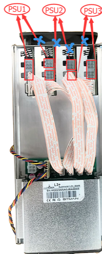
Figure 2-2. PCI-E Connectors - Incorrect Connection
